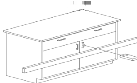
Figure 8. Base Cabinet Door and Drawer Pull Horizontal Load Test Configuration
