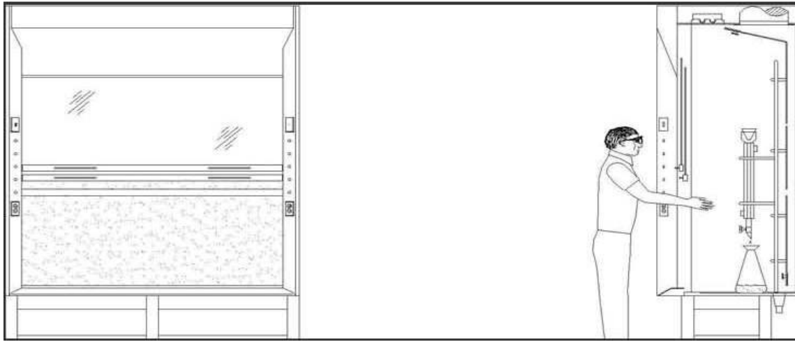
Fig. 7 Typical View of Distillation Fume Hood
